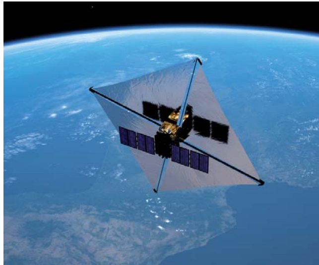
ADEO-Bremssegel, Foto: Plattform P200 (QinetiQ Space), De-Orbit System (HPS GmbH)
